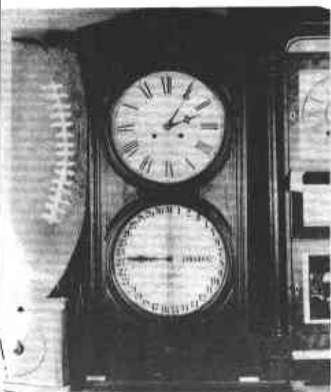
Very large so-called bank model, also known as #3 regulator, weight driven carrying serial number 1528. Made under Horton patents of April 18, 1865 and August 28, 1866
