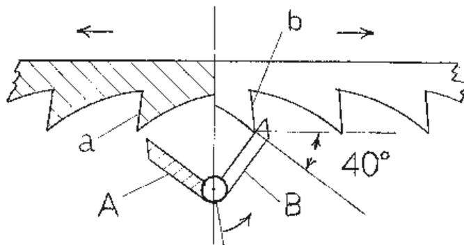
Figure 21, left. Verge escapement used in lantern clocks and bracket clocks 1650-1750 (shown inverted for comparison with Figure 22).
