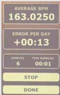
**ClockMaster** is a new digital smartphone app for measuring and regulating mechanical pendulum clocks. The app uses a microphone to capture the audible ticks of the clock escapement and pendulum to determine the beats per minute and the rate of error in seconds per day fast or slow.
