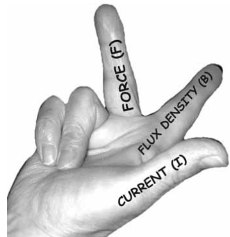
Figure 3, below. Figure to illustrate the right-hand rule to find the direction of the force due to a current in a magnetic field.
